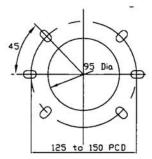
Drill & Tap 2 x M8 holes on the horizontal centre line or 4 x M8 holes at 45 degrees
