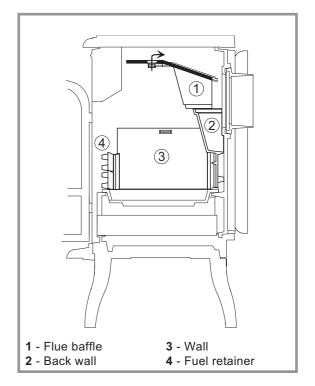
Figure 8 Put back into position the elements
