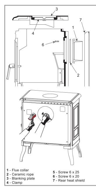
Figure 3 - Rear flue outlet
