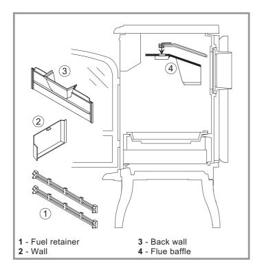
Figure 7 Removing the flue baffle
