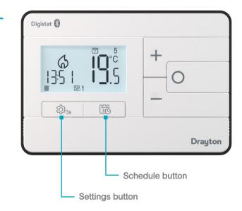
If you are using the dual-channel RF902 you can toggle between heating and hot water by pressing briefly the settings button and using the up and down buttons to select heating or hot water mode. In hot water mode ON/OFF times can be adjusted (Settings Button - Page 14)
