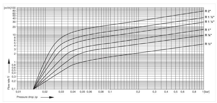
$Fig.\ 3\ Pressure\ drop\ within\ the\ valve\ in\ dependency\ of\ the\ flow\ rate\ and\ the\ used\ connection\ size$
