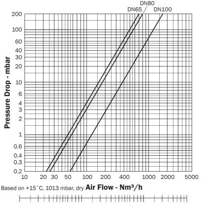
Based on f = 1.24 Natural Gas Flow - Nm<sup>3</sup>/h
