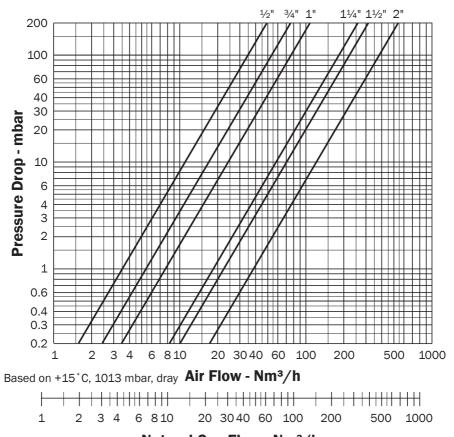
Based on f = 1.24 Natural Gas Flow -  $Nm^3/h$
